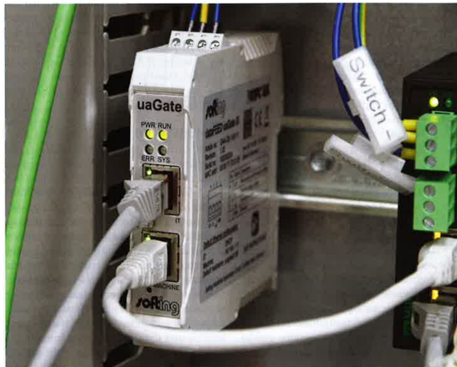
Open, platform-independent OPC UA technology offers straightforward networking at a local and a global level, along with allowing secure data traffic through a firewall.
