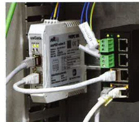
Physically separate network interfaces in the uaGate SI Gateway offer maximum protection from attacks.
